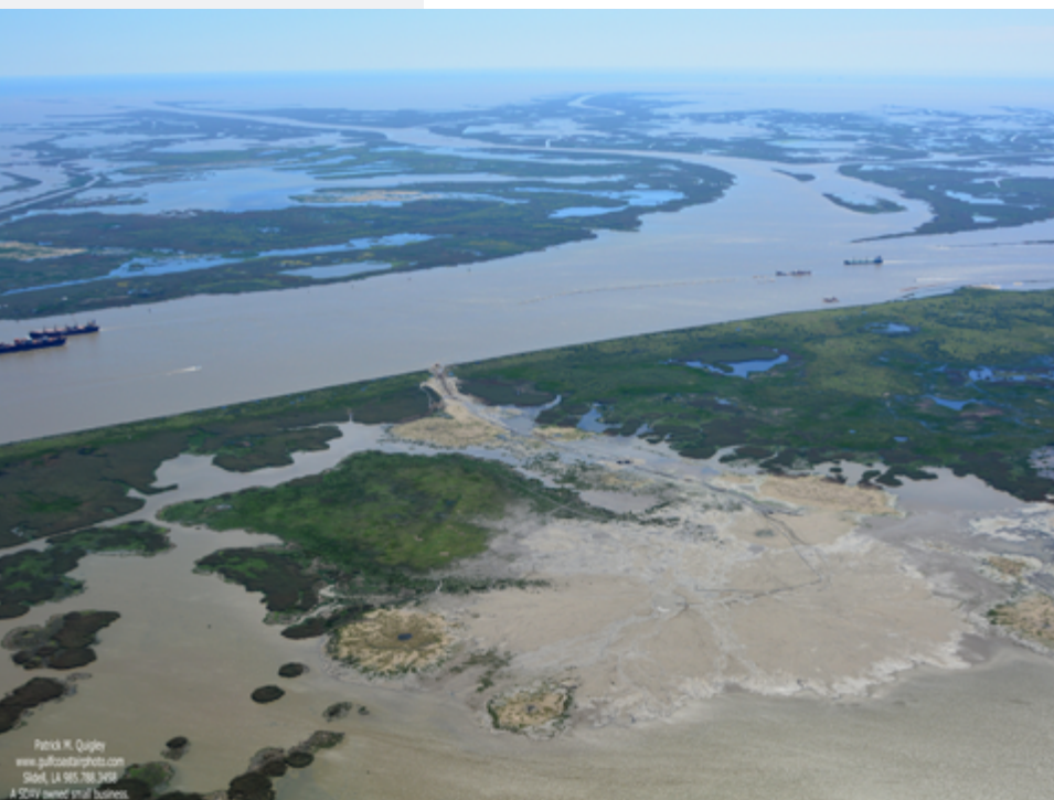
A cutterhead dredge works just above the Head of Passes with ship traffic passing. Also shown are areas of new land being created by the beneficial use of dredged material in the bottom half of the photo.
