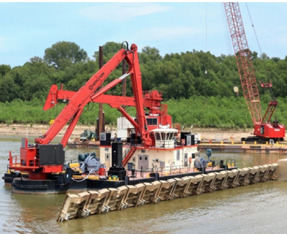
One of two Olmsted Lock and Dam Wicket Lifters were delivered to the Corps of Engineers by Conrad Shipyard.
